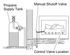
Figure 16 - Checking Gas Joints
